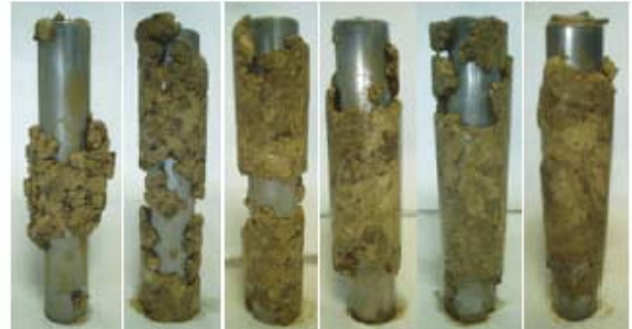
Figure 2: Arne clay accretion profile over time ( 5, 10, 20, 40, 60 and 80 minutes).
