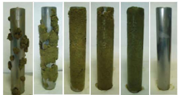
Figure 4: Lillebaelt clay accretion profile over time ( 5, 10, 20, 40, 60 and 80 minutes).
