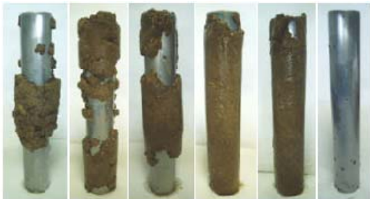
Figure 1: Accretion profile over time at 5, 10, 20, 40, 60 and 80 minutes.
